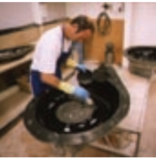
The Nautilus™ shell is all hand-made, except for two parts: the internal spiral which sits inside the shell's gleaming exterior and a dual-purpose bolt, which anchors the shell to its plinth and provides a conduit for wiring from the power amplifiers.
