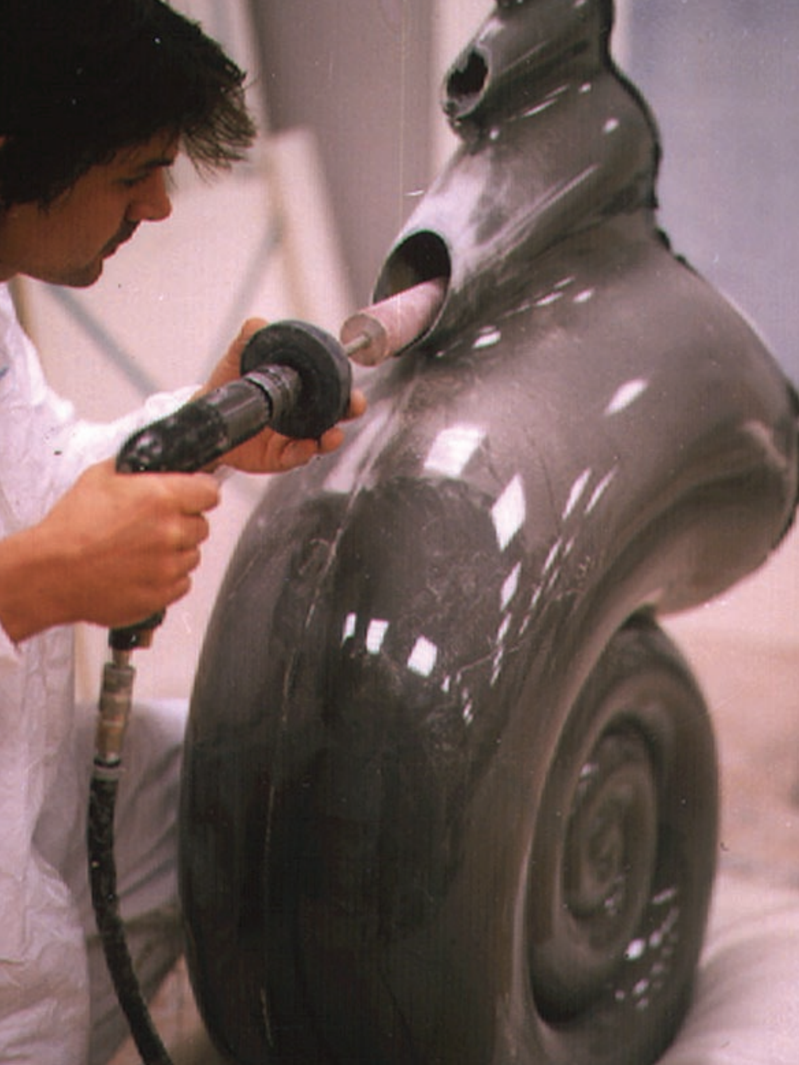
The Nautilus™ shell is all hand-made, except for two parts: the internal spiral which sits inside the shell's gleaming exterior and a dual-purpose bolt, which anchors the shell to its plinth and provides a conduit for wiring from the power amplifiers.
