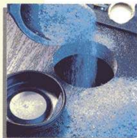
Filling the sand chamber
